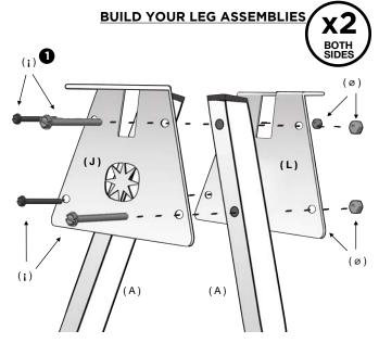
Attach J-Brackets to each vertical leg with screws and nuts.
