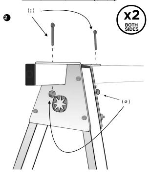
Slide the Hanger-Bar (B) through the openings on both leg assemblies. Line up the pre-drilled holes of the Hanger-Bar with the corresponding holes in the J-Harvest Brackets. Partially tighten.
