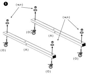
Begin by attaching all four castors (O) to the two Wheel-Bars (A). Thread the castor bolt through **both** holes on each end of the Wheel-Bars and fit the castor washer and nut on the top end of the castor bolt (as pictured) tighten by hand.
