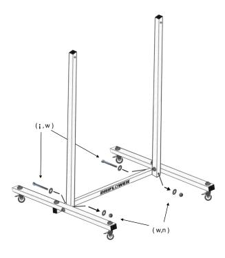
\*\* IMPORTANT NOTE: MAKE SURE THE PRE-DRILLED HOLES IN THE VERTICAL POSTS ALIGN WITH THE HOLES IN THE CROSS-BAR OF THE BASE-ASSEMBLY.
