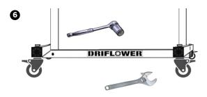
Once all parts have been connected, tighten each bolt and nut using the appropriate wrenches and drivers.
