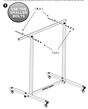
Attach the Hanger-Bar to the top of the Vertical Posts using 3" hex bolts (¥), washers (w) and 1/2" hex nuts (n).
