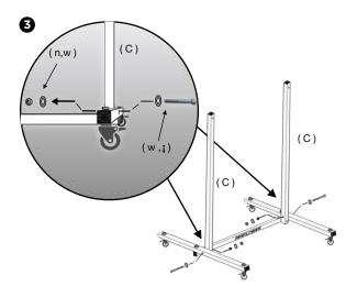
\*\* IMPORTANT NOTE: VERTICAL POSTS HAVE TWO SETS OF HOLES ON THE BOTTOM OF EACH POST THAT ALIGN WITH THE HOLES OF YOUR BASE-ASSEMBLY.
