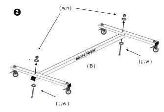
Attach both Wheel-Bars **above** the center holes of the Cross-Bar using 3 3/4" hex bolts (i), washers (w) and 1/2" hex nuts (n) on each side. Tighten by hand.
