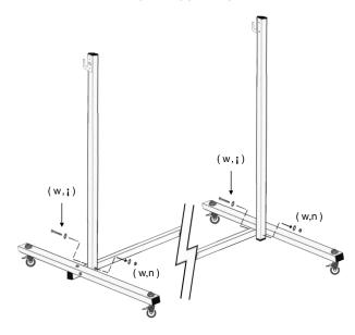
\*\* **IMPORTANT NOTE**: MAKE SURE THE PRE-DRILLED HOLES IN THE VERTICAL POSTS ALIGN WITH THE HOLES IN THE CROSS-BAR OF THE BASE-ASSEMBLY.
