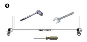
Once all parts have been connected and you have verified the J-Brackets are centered over the Cross-Bar, proceed to tighten each bolt and nut using the appropriate wrenches and drivers.
