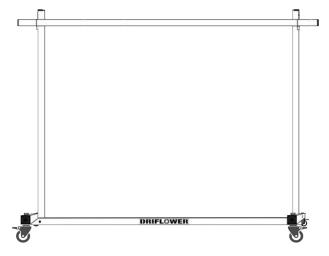
When all connections have been tightened, the final step is to place your Aluminum Stick in the J-Brackets so that the stick is evenly distributed with equal overhang on each end. This helps stabilize the bar seated in the J-Brackets.
