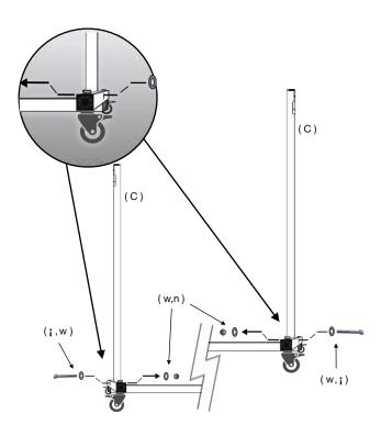
\*\* IMPORTANT NOTE: VERTICAL POSTS HAVE TWO SETS OF HOLES ON THE BOTTOM OF EACH POST THAT ALIGN WITH THE HOLES OF YOUR BASE-ASSEMBLY.
